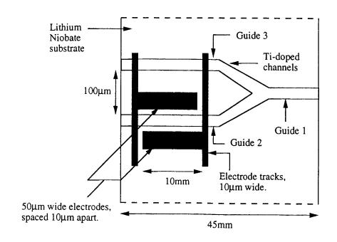
Fig. 1. Schematic of a Y-branch waveguide laser device.
