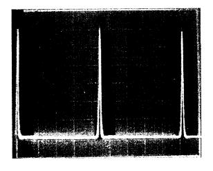
Fig. 3. Oscilloscope trace of one Q-switched pulse.
