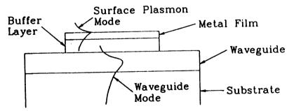
FIG 1: Waveguide-coupled surface plasmon resonance sensor.
