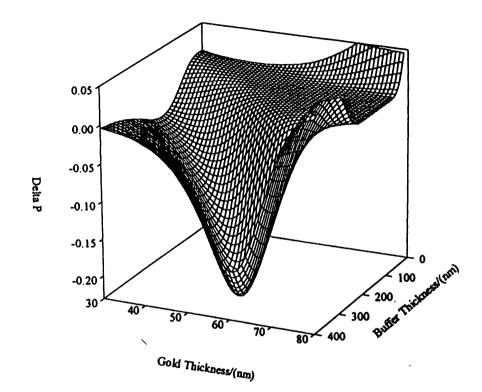
System Parameters:-Superstrate Index=1.33 Film Index=1.47 Film Thickness=7nm Film Length=1.5mm Buffer Index=1.29 Guide Index=1.47 Guide Depth=2µm Substrate Index=1.46 \(\lambda=639nm\)
