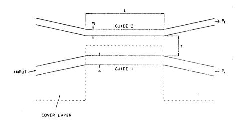
FIG 3: Lateral directional coupler sensor.
