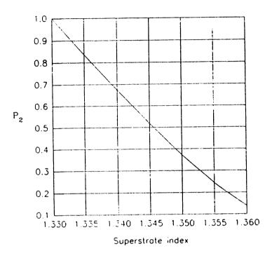
FIG 4: Normalised power output from guide 2 of a lateral coupler as a function of superstrate index.  $w_1 = 3 \mu m$ ,  $w_2 = 2.75 \mu m$ ,  $s = 10 \mu m$ , BGG31 substrate, MgF<sub>2</sub> cover layer.
