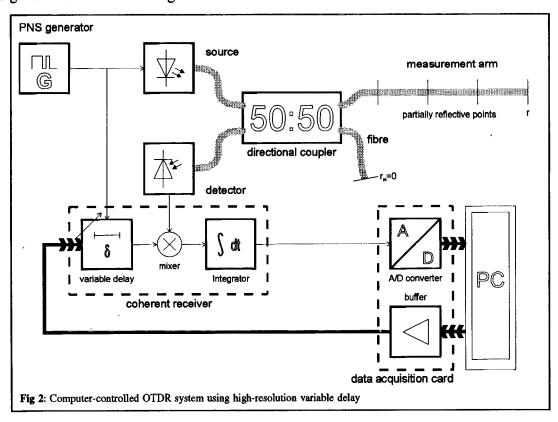
In the system in Fig 2, a digital signal is transmitted by a 780 nm CD-type laser and received by a fast silicon photodiode. Integrated circuits for fast telecommunication links support the electro-optic design.<sup>7</sup>
