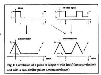
For many sensor systems, a typical OTDR spatial resolution of 1-10 m is sufficient, but there is a need to monitor each reflective point with a range accuracy below 1 mm. Our current technique overcomes this problem by interrogating the slopes of the correlation peak.<sup>††</sup> These slopes (bottom of Fig 1) are normally not used because receivers of OTDRs do not allow a continuous sweep of the output.
