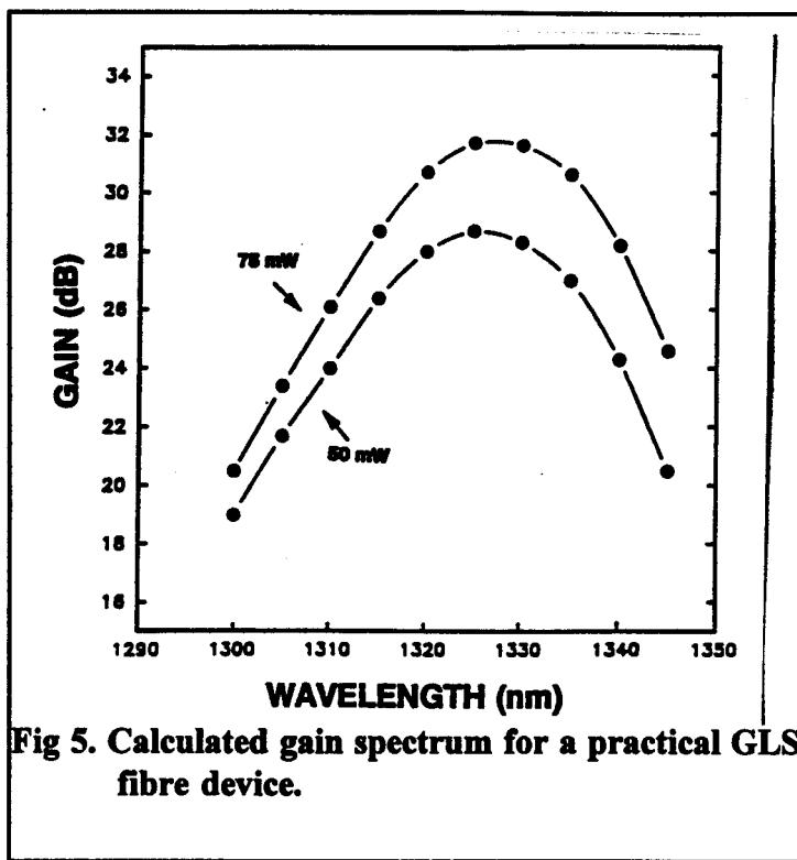
Fig 5. Calculated gain spectrum for a practical GLS fibre device.
