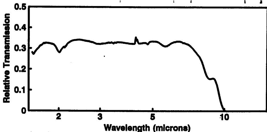
Fig.2 Transmission Spectrum of doped GLS glass by FTIR spectroscopy
