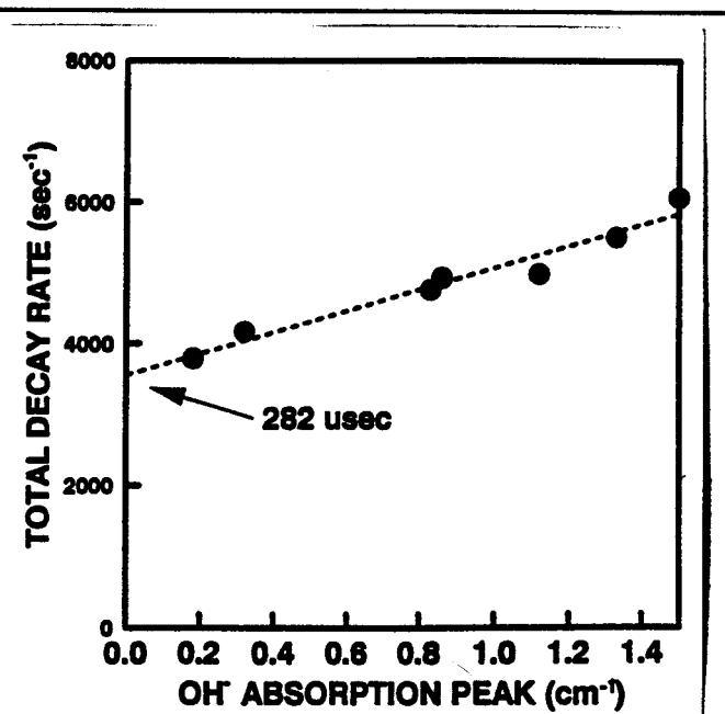
Fig.4 Influence of  $\text{OH}^-$  on measured lifetime for GLS glass
