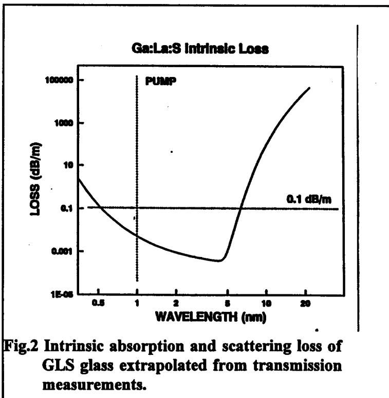
Fig.2 Intrinsic absorption and scattering loss of GLS glass extrapolated from transmission measurements.
