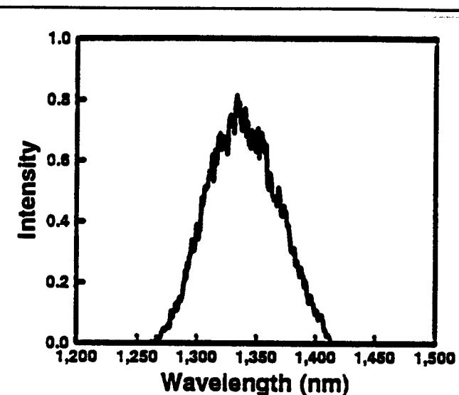
Fig.3 Fluorescence spectrum of  $\text{Pr}^{+3}$ -doped GLS glass pumped at 1.02 microns.
