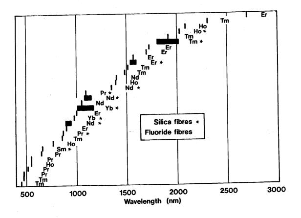
Fig 1 Fibre laser wavelengths
