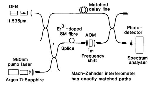
Figure 1. Matched-path Mach-Zehnder Interferometer used to measure spectral broadening.
