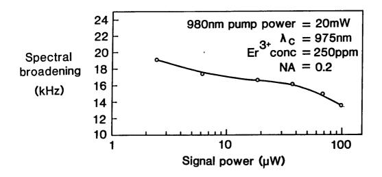
Figure 3. Variation of spectral broadening with signal power.
