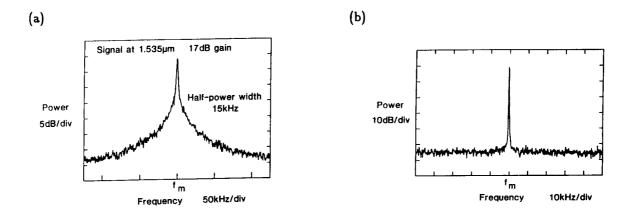
Figure 2. (a) Measured power spectral density. (b) Mach-Zehnder response with amplifier replaced by un-doped fibre.
