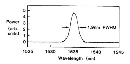
Figure 2 Super-radiant output spectrum  $\hbox{\it @ 1.535}\mu\hbox{m. 0.2nm resolution.}$
