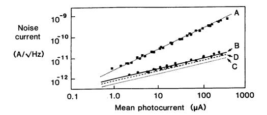
Figure 3 Noise characteristic without compensation (squares) and with compensation (circles).
