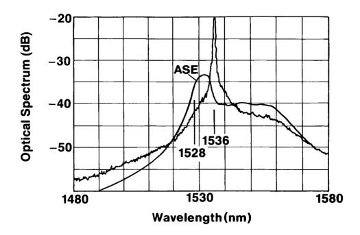
Fig. 2: Erbium-doped fiber amplifier output spectra with and without the 1536 nm signal. ASE: amplified spontaneous emission.
