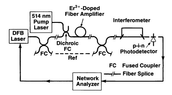
Fig. 1: Experimental set-up for measuring the response of an erbium-doped fiber amplifier. The two paths of the interferometer refer to the fast and slow axes of the birefringent fiber.
