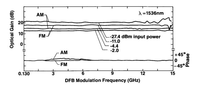
Fig. 3: Erbium-doped fiber amplifier response versus DFB modulation frequency, for AM and FM signals at 1536 nm.
