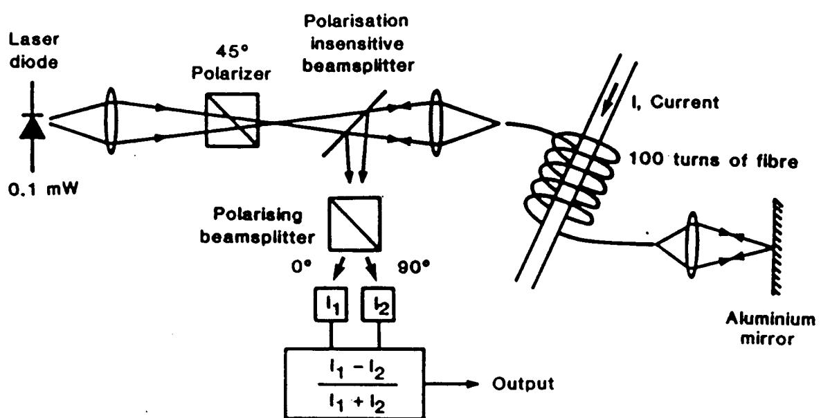
Figure 1. Schematic diagram of the fibre current monitor
