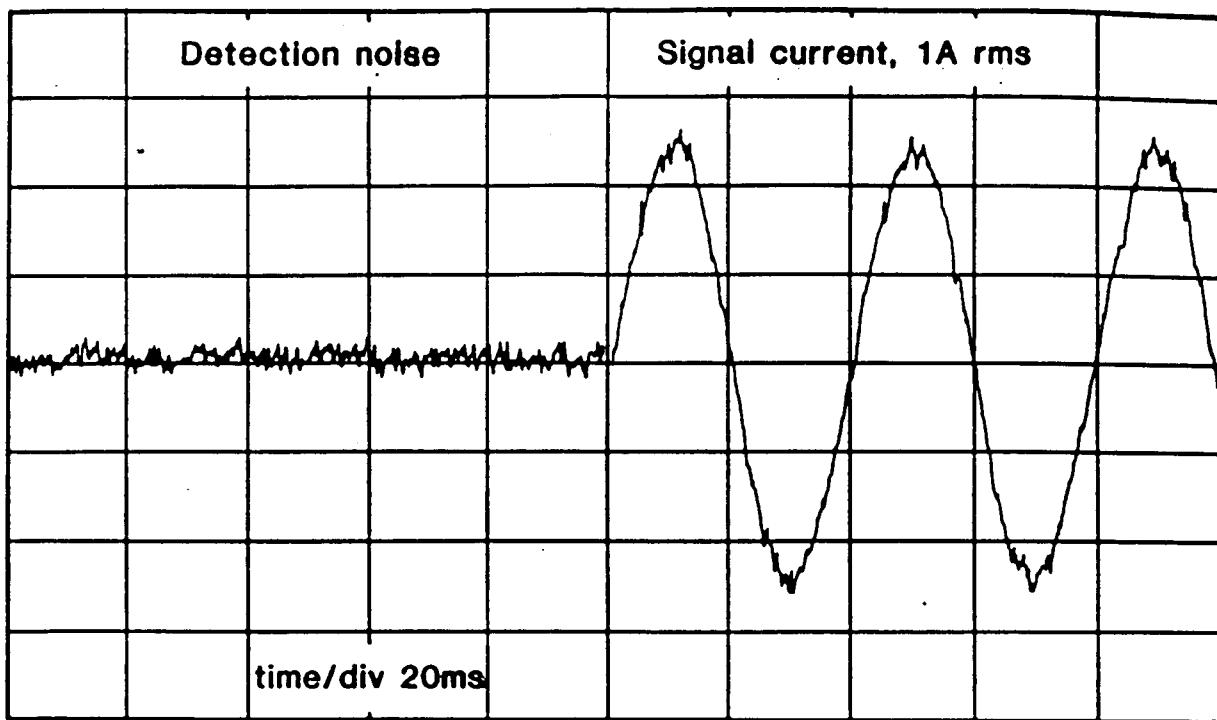
Figure 2. Oscilloscope trace of the sensor noise output and response to a 1A rms signal current at 25Hz.
