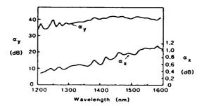
5. Measured spectral attenuation of x and y-polarised modes for polariser B. Metal length is 5cm.
