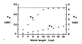
4. Measured attenuation of x and y-polarised modes for polariser A for various lengths of the metal sector.
