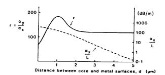
2. Calculated ratio of attenuations of x and Y-polarised modes as a function of core-to-metal distance d. Also shown is the insertion loss per unit length of the x-polarised mode.
