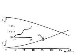
Power in each of the orthogonally polarised modes as a function of the number of turns, N, for the case where  $\mathbb{E}_{\chi}(0) = 1$ ,  $\mathbb{E}_{\chi}(0) = 0$ . Coil diameter 15mm.
