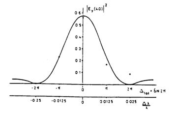
Fig. 4 Power, E (z=40 turns) 2, converted to the orthogonal mode for 15mm dia. coil as a function of the total mismatch. Individual point points were obtained by applying tension to the coil to vary the fibre birefringence. Lower abscissa shows the spectral response that would be obtained if the coil were used as an optical fibre.
