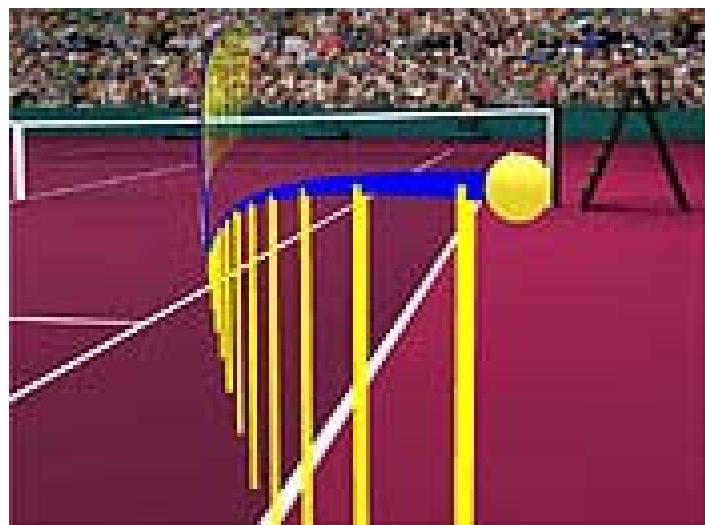
The system uses five cameras at in different locations around the court to observe the path of the ball as it flies through the air. The information from these cameras can then be combined using computer software to make a 3D model of the flight of the ball, which is accurate to within 2 to 3 millimetres. The software can create the model within 2 seconds of the end of the shot – easily fast enough for most uses.
