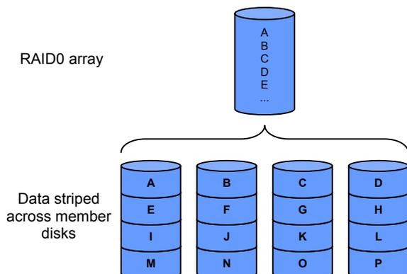
In a RAID0 array the data is broken down into small pieces, called strips, which are then distributed across the member disks.
