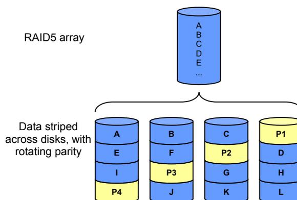
The optimal storage efficiency, reasonable performance, and fault tolerance means that RAID5 is the most commonly used RAID level.
