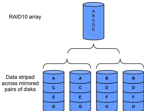
It is suitable for similar applications to RAID1, where data reliability and fault tolerance are more important than cost. An additional benefit of RAID10 over RAID1 is increased performance.
