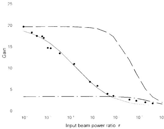
Fig. 2. Two-beam coupling gain as a function of the input power ratio for the case of beams focussed to  $2w_0 = 400 \mu\text{m}$  in diameter in a bulk crystal  $\beta = 0^\circ$ ,  $\theta = 24^\circ$ ,  $IL = 3$ ,  $a = 11$  ●: experimental data, solid line: theoretical fit with the nonlinear response empirical correction function, dashed-dot line: standard theory curve for the value of  $IL = 1.2$ , (value expected from the standard theory) dashed line: standard theory curve for  $IL = 3$ .
