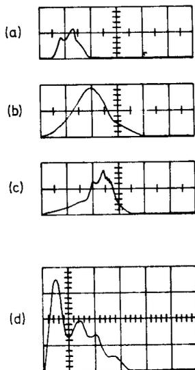
Fig. 2. (a) Dye laser output ( $\approx 740 \text{ nm}$ ). (b) Ruby laser output. (c) Time-overlap of dye and ruby laser outputs. (d) Difference-frequency signal. Time bases: (a) - (c) 10 nsec/div; (d) 50 nsec/div.
