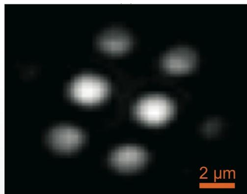
Optical image is distorted by diffraction from 2 $\mu$ m holes – pinhole and membrane are not flush.
