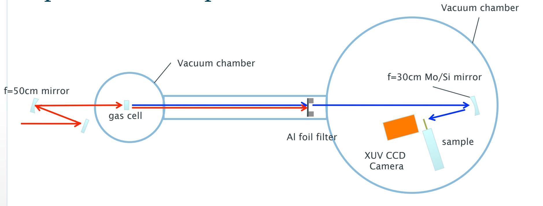
XUV source: HHG in Ar-filled capillary or cell, peaked at  $\sim 29$  nm
