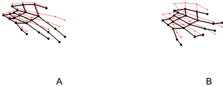
Figure 14 Operating deflection shapes in condition #7 (palm in contact with the vibrating plate with no contact at the fingers) at 22 Hz (A) and 46 Hz (B) : — reference position; —●—●— deflection.
