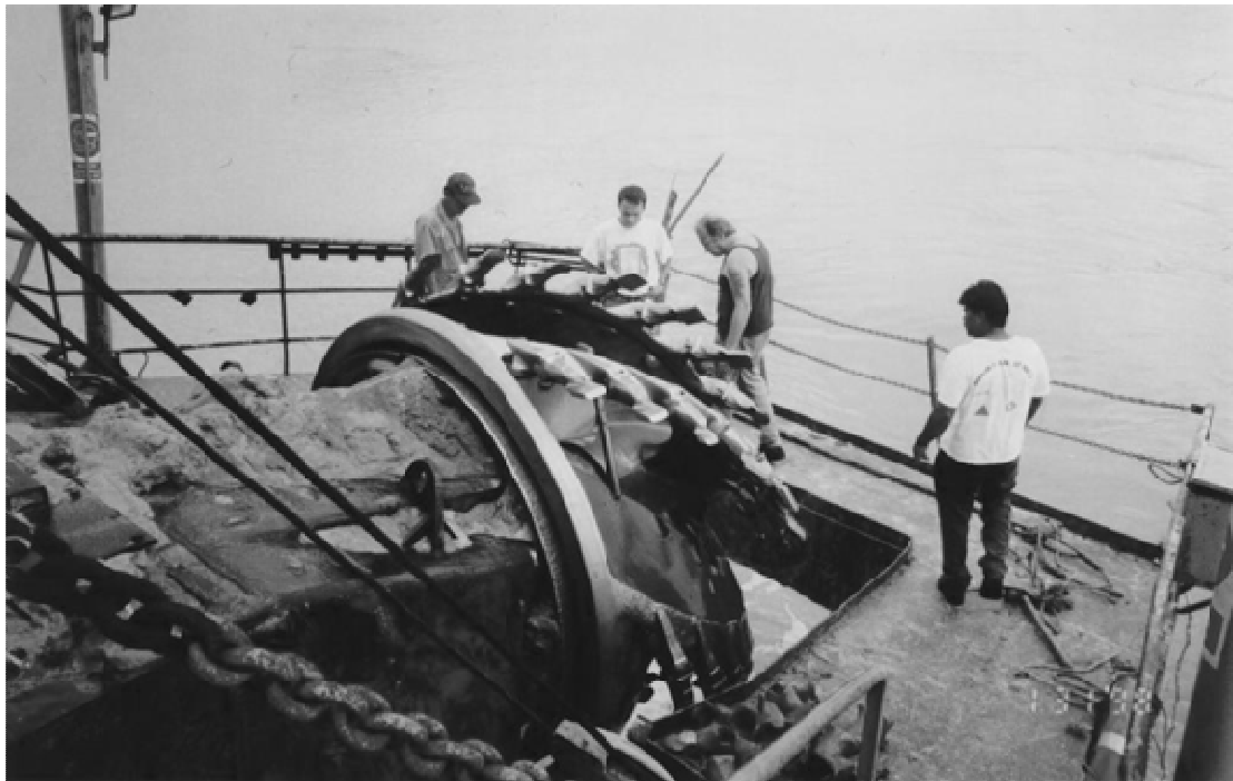
Figure 2.2 Routine inspection of a sand/clay cutterhead.
