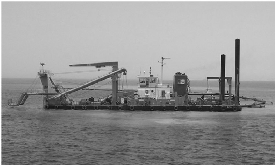
Figure 1.1 Medium size cutter suction dredger (Courtesy Gulf Cobla L.L.C.).
