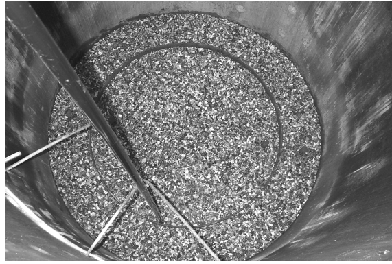
Figure 5.1 Gravel layer installed at the base of the compression cell ready for waste sample to be loaded. The tube on the left hand side of the photo is the extensometer tube for mounting magnets to assess differential settlement
