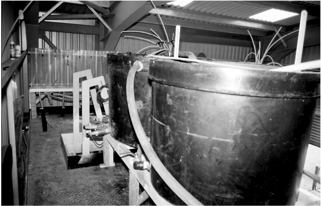
Figure 3.5. Individual Perspex header tanks (left background) for leachate supply for horizontal flow connected to main header tanks (right foreground)
