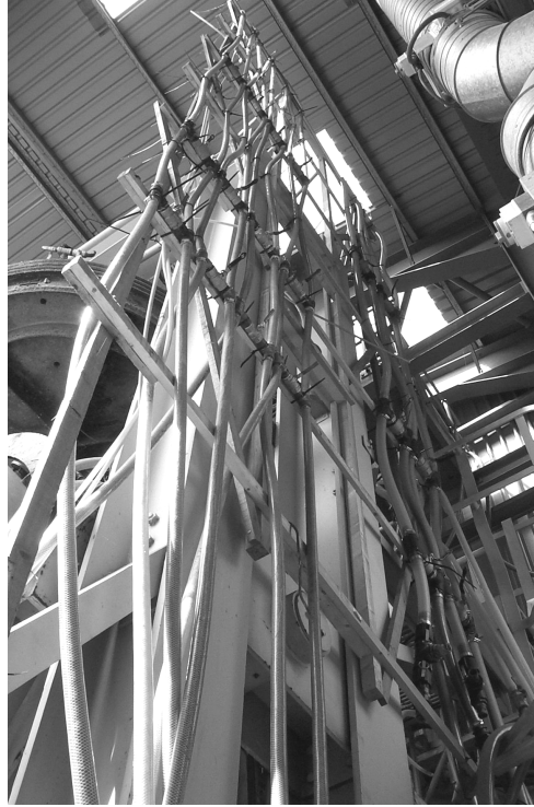
Figure 7.3 The outlet valves and pipes mounted on the side of the compression cell
