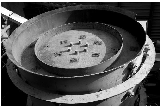
Figure 8.14 Compression cell bottom platen (in fully extended eject position) showing top surface normally covered by the bottom gravel layer. The dividing ring protrudes through the gravel layer into the waste sample
