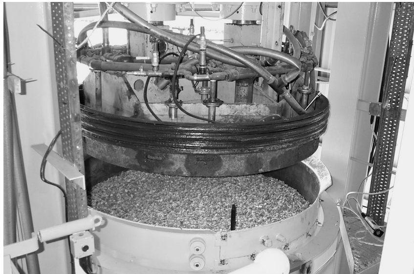
Figure 3.2. Top platen showing the stack of three inflatable seals added to allow horizontal flow tests to be carried out
