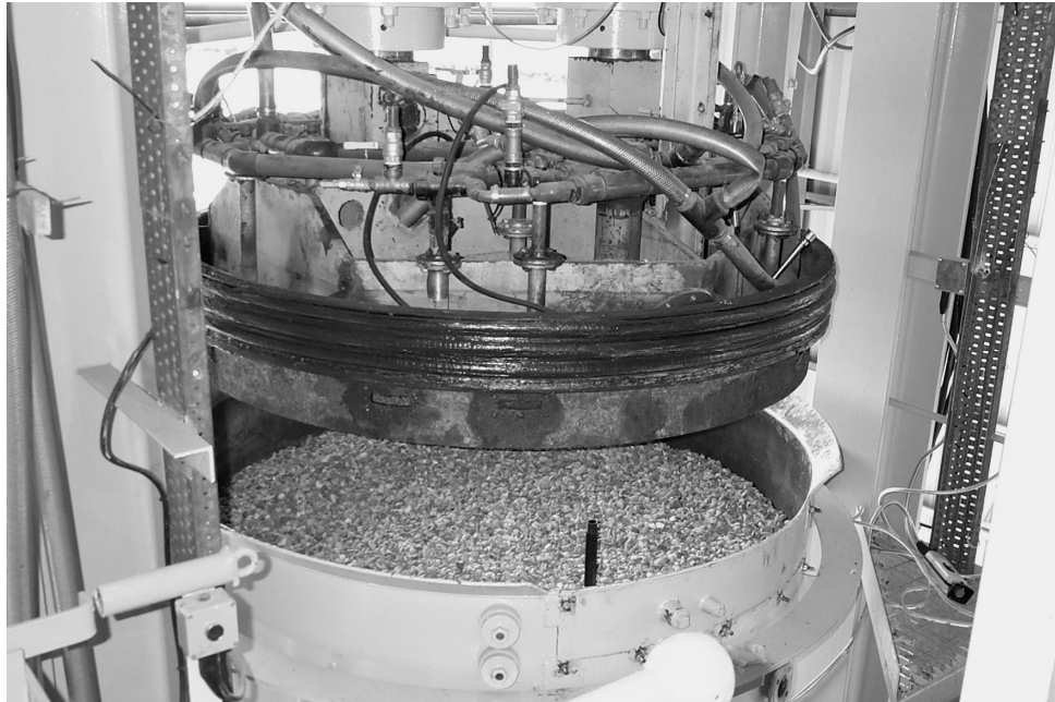
Figure 5.4. Top gravel layer installed prior to lowering the top platen
