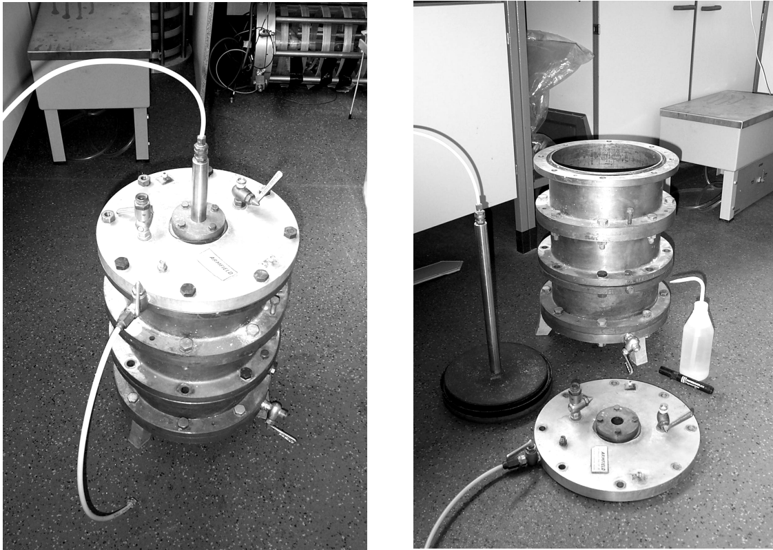
Figure A8. Rowe cell design using o-ring seal in top plate assembled (left) and disassembled (right)
