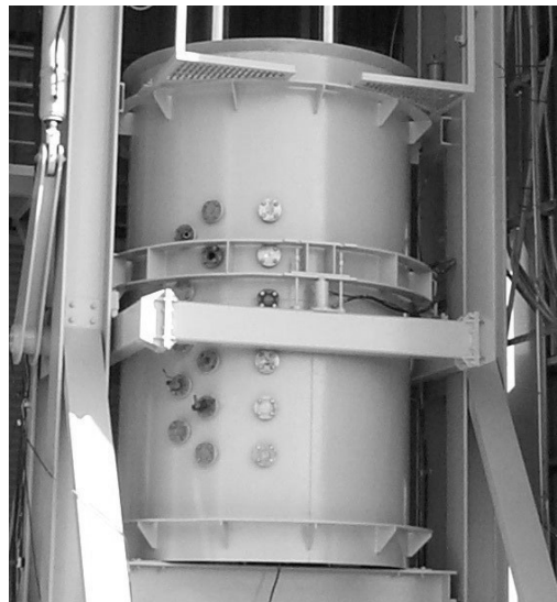
Figure 3.4. Close up view of horizontal flow outlet 'E' ports (two columns on left), and piezometer monitoring 'C' ports (right) for the outlet region
