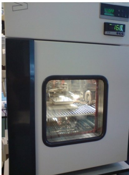
Figure 5.4.1 Picture of the WKL environmental chamber used to control temperature and relative humidity.
